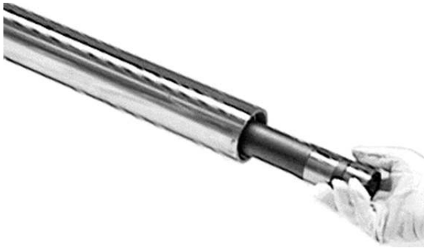
Figure 8-4. Tilting the Body/Anvil to Access the Striker.
