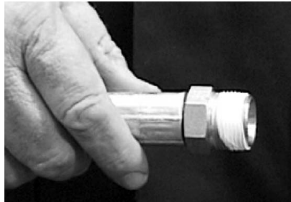
Figure 9-24. Apply Teflon Tape to Hose Fitting.
