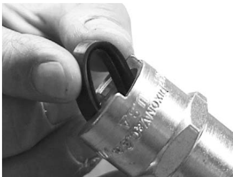
Figure 8-8. Remove Gasket from Coupling Socket.
