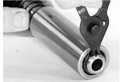
Figure 8-13. Remove Valve Retaining Ring from Valve Stem and Valve.
