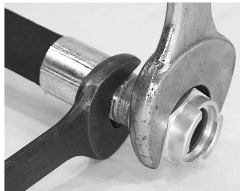
Figure 11-2. Remove Whip Hose from Q.D. Socket
