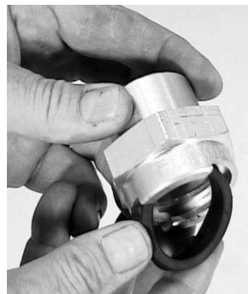
Figure 11-3. Remove Q.D. Gasket
