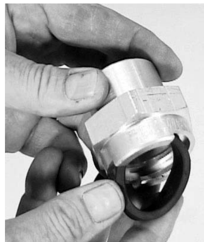
Figure 8-9. Remove Gasket from Coupling Socket.
