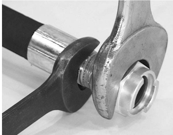
Figure 8-8. Remove Coupling Socket from Whip Hose.
