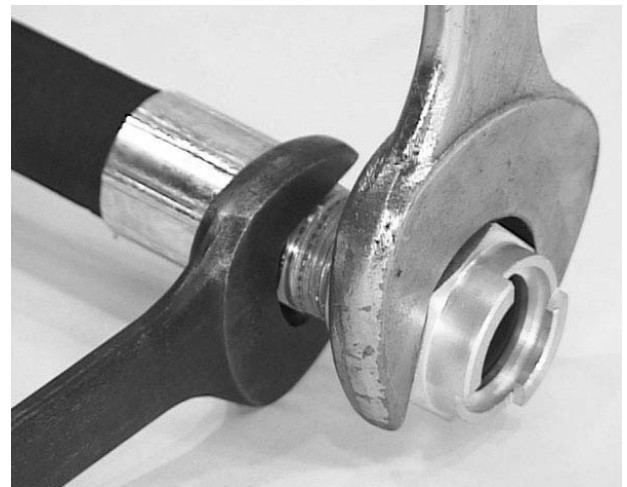
Figure 9-10. Secure Whip Hose to Q.D. Socket.
