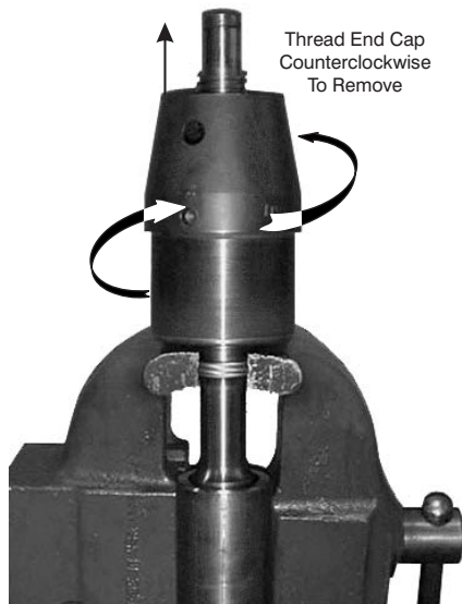
Figure 8-9. Remove the Hose Socket and Whip Hose from the Valve Stem.
