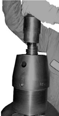
Figure 11-21. Align Valve Nut on Valve Stem.
