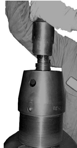
Figure 9-19. Align Valve Nut on Valve Stem.
