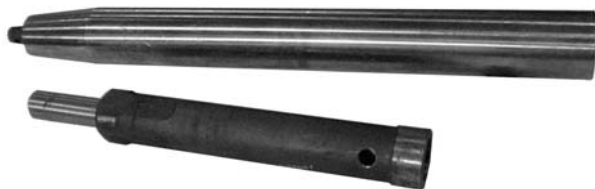
Figure 8-6. Striker Removed from Body/Anvil.
