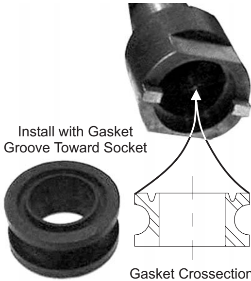
Figure 9-8. Install Gasket in Q.D. Socket.
