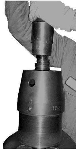
Figure 11-4. Thread the Valve Nut from the Valve Stem.
