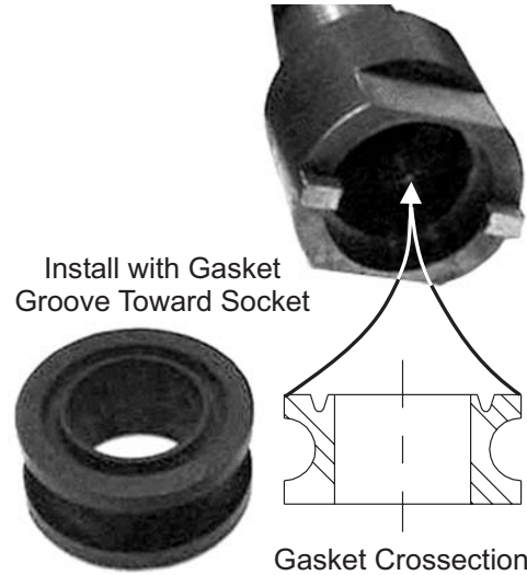
Figure 11-13. Install Gasket in Q.D. Socket.
