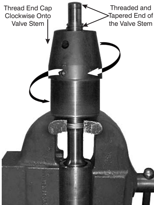
Figure 9-18. End Cap Threaded onto Valve Stem
