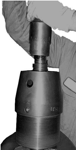
Figure 8-8. Thread the Valve Nut from the Valve Stem.
