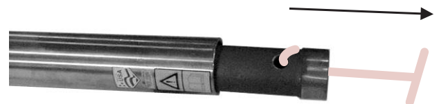
Figure 8-4. Access the Striker with a Hook.
