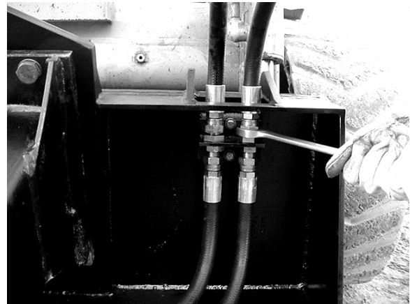
Figure 7-11: Connecting Hydraulic Lines to Bulkhead Adapter
