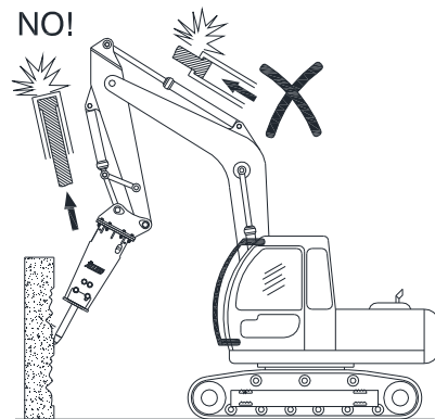
Fig 6-9 Do Not Operate With Cylinder at Stroke End
