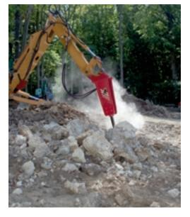
One or more of over 2,500 customized hydraulic kits from Allied provide components for mounting the Model AR 85B on backhoes and excavators. The Model AR 85B requires 16 to 26 gpm at 1,600 to 1,890 psi and it breaks at a rate of 500 to 900 blows per minute.
