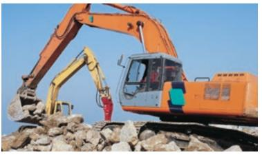
One or more of over 2,500 customized hydraulic kits from Allied provide components for mounting the Model AR 95B on backhoes and excavators. The Model AR 95B requires 18 to 33 gpm at 1,740 to 2,030 psi and it breaks at a rate of 350 to 700 blows per minute.
