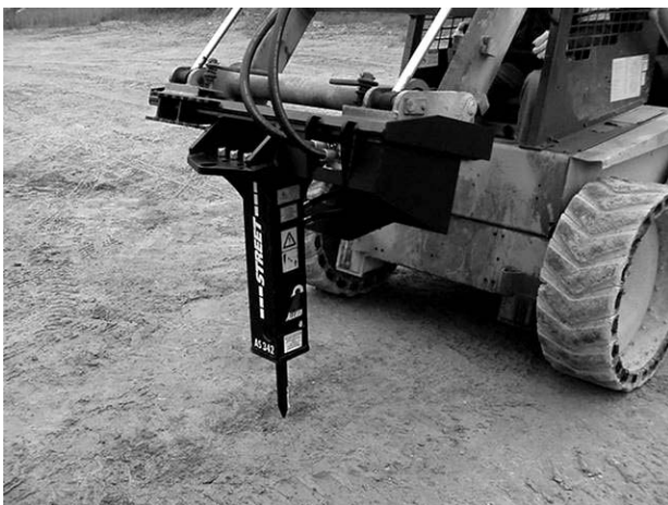
Figure 8-3. Keep Contact Pressure on Tool
