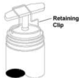
Fig. 6-2 Retaining Clip Attached to Follower Rod
