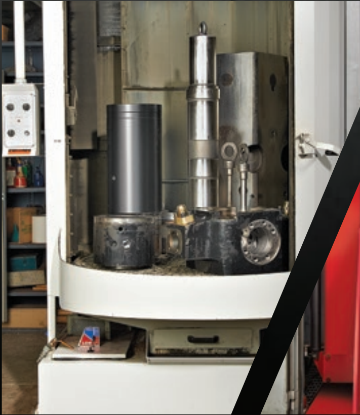
The front-load automatic parts washer used for the REMAN Program with a pump capacity of 200 gpm at 50 psi cleans both larger parts up to 60" high and smaller parts contained in a small parts basket.
