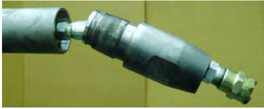
Figure 11-6 Tail Adapter, Whip Hose and Q.D.
