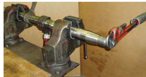
Figure 10-4 Tighten Nose Cap
