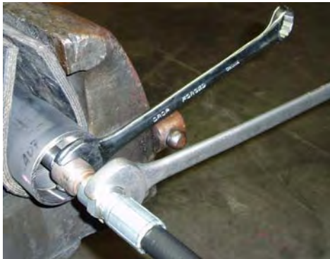
Figure 10-11 Whip Hose Removal/Installation
