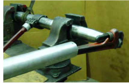
Figure 10-3 Loosen Nose Cap.
