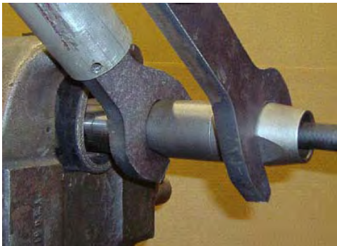
Figure 10-8 Secure Hole-Hog for Tail Adapter removal
