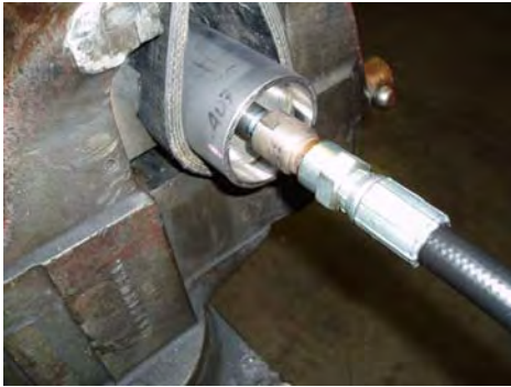
Figure 12-13 Press Valve Stem to expose Thread Adapter.
