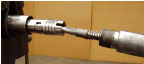
Figure 12-20 Prepare Body/Anvil and Tail Assembly for Installation
