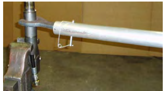
Figure 11-5 Secure End Cap for Disassembly
