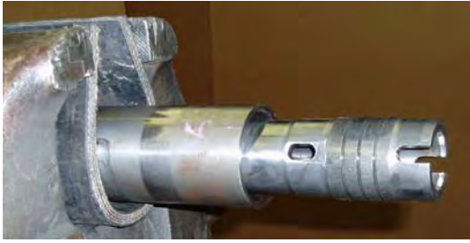
Figure 12-19 Inserting Striker into Body/Anvil
