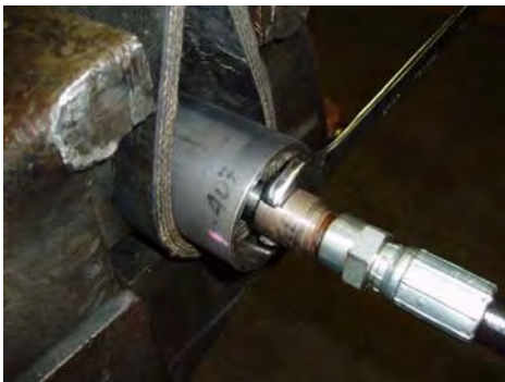
Figure 12-14 Hold Thread Adapter in Position
