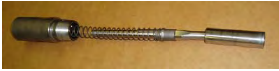
Figure 12-11 Valve Spring, Stem, and Guide
