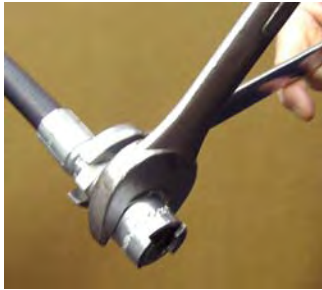
Figure 12-16 Secure the Q.D. Fitting to the Whip Hose Fitting
