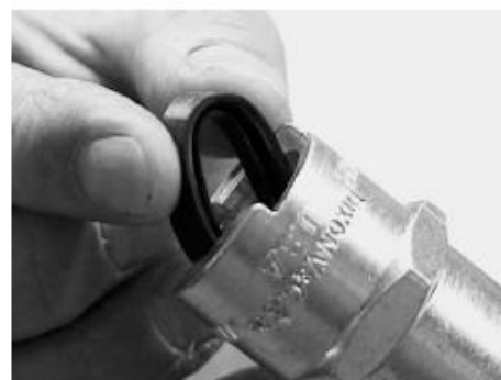
Figure 10-7 Install New Gasket
