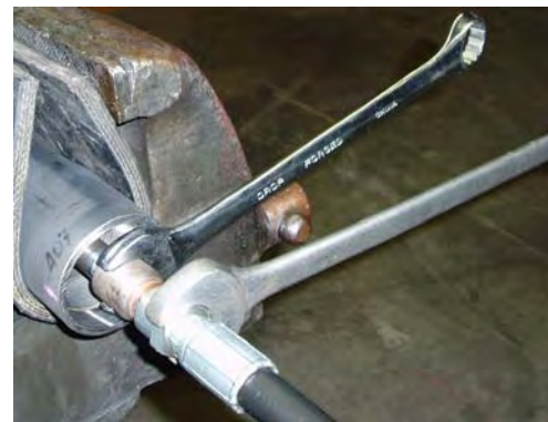
Figure 12-15 Tighten Whip Hose
