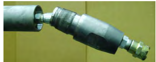
Figure 12-22 End Cap and Tail Adapter
