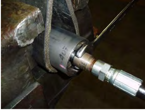
Figure 10-10 Secure Thread Adapter for Whip Hose Removal/Installation
