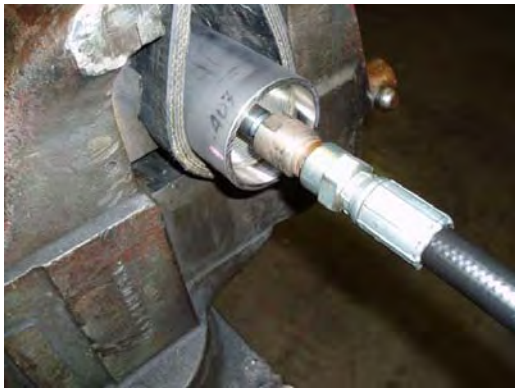
Figure 11-7 Press Valve Stem to expose Thread Adapter
