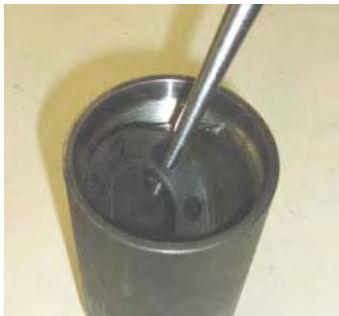
Figure 11-17 HH79 Shock Absorber and Pry Bar
