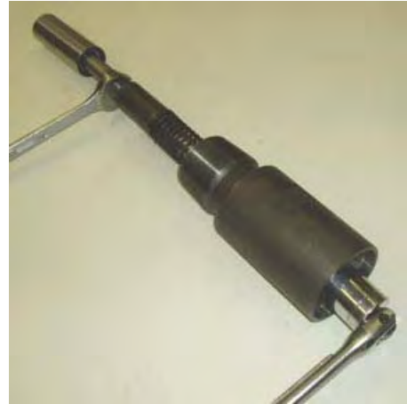
Figure 12-12b HH79 Tighten Thread Adapter to Valve Stem.
