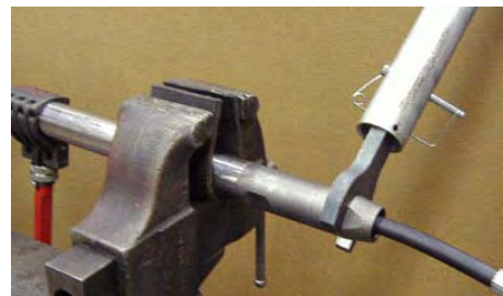
Figure 12-24 Tighten End Cap and Tail Adapter
