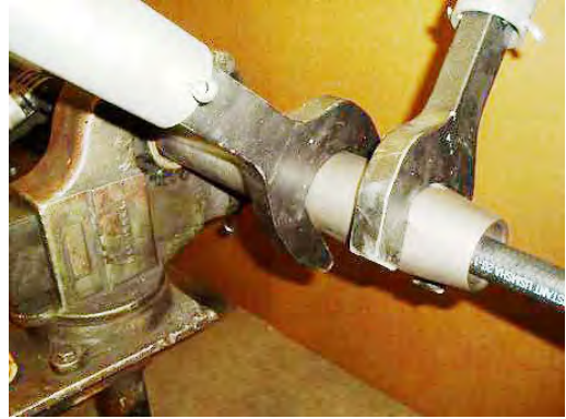
Figure 10-13 Tighten Tail Adapter to End Cap
