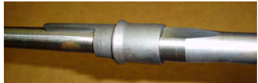
Figure 12-10 Valve Fingers installed to Valve Stem Assembly
