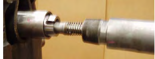
Figure 12-21 Insert Valve into Body/Anvil and Striker
