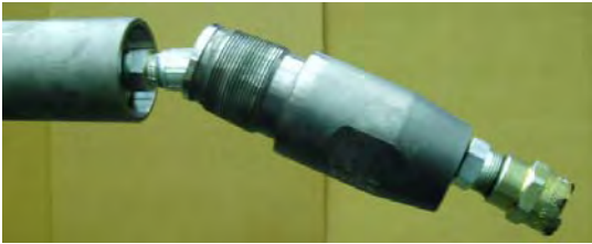
Figure 10-12 Tail Adapter and End Cap
