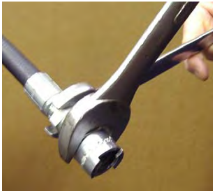
Figure 10-5 Q.D. Fitting and Whip Hose
