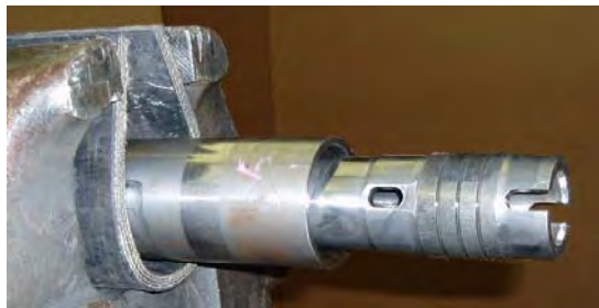
Figure 11-4 Removing Striker from Body/Anvil
