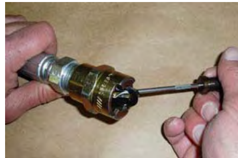
Figure 10-6 Q.D. Fitting Gasket
