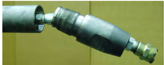
Figure 10-9 Unthread Tail Adapter and slide over Whip Hose
