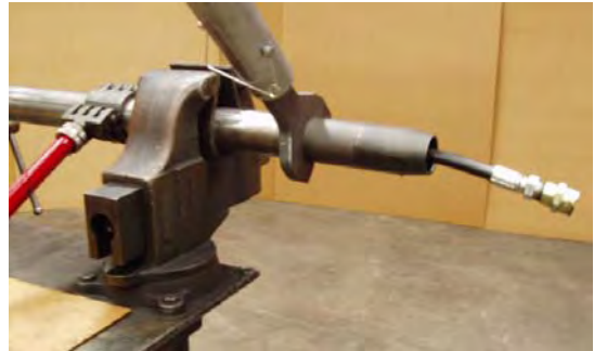
Figure 11-2 Loosening of Tail Assembly
