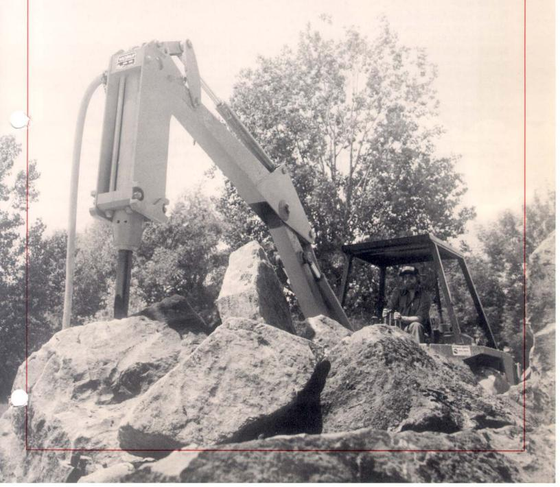
llied Ho-Rams are economical and profitable additions to rental center and contractor fleets. They are easily installed on most backhoe/loaders and excavators. When powered by air compressors, Ho-Rams provide an efficient means of demolishing rock, concrete, brick, and more.
