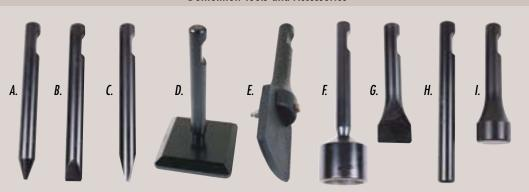
A. The Conical Tool\* is extremely useful when solid materials are being broken. With no seam or relieved sections to break toward, the "pencil" point easily penetrates materials because its shape allows trapped dust to escape on all sides of the tool.
