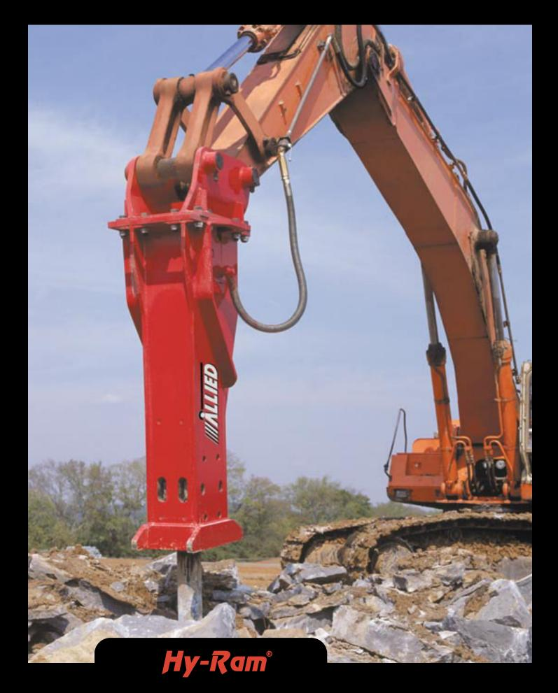
Allied's all new Model 797CS and Model 797CS G hydraulic impact hammers
