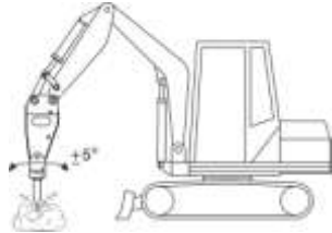
Fig 5-3 Tilt the Breaker No More Than 5°
