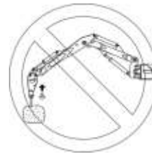
Fig 5-6 Do Not Pound the Breaker at the Material
