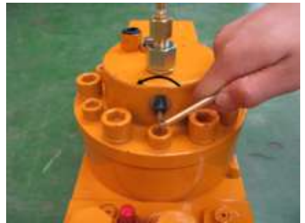
6. Open needle pin. (If equipped) Turn counter-clockwise.
