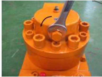
2. Remove protective cap from needle pin. (Not equipped on all models)
