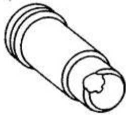
Fig 6-8 Damaged Piston Impact Face
