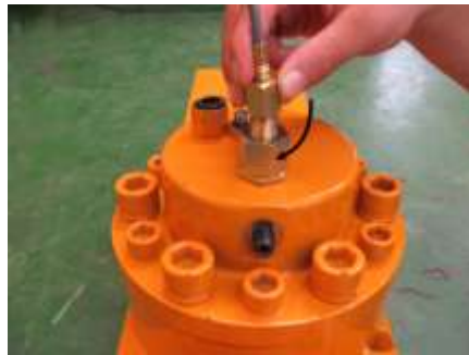
5. Attach other hose end to charging adaptor.
