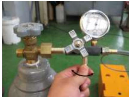
8. Wait 3 minutes minimum for gas temperature to stabilize. Monitor gage while opening bleed valve for final pressure.
