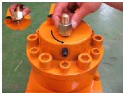
11. Unthread charging adaptor from inlet.
