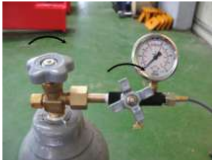
4. Attach 3-way valve to gas bottle. Attach hose to 3-way valve.
