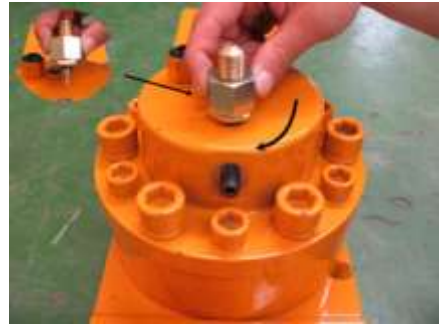
3. Thread charging adaptor into the inlet. NOTE: Must install without hose attached.
