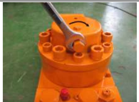
12. Reinstall threaded plug and cap.
