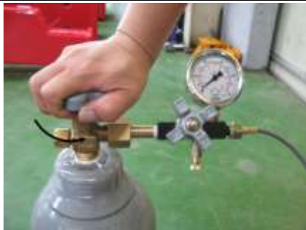
7. Slowly open gas bottle valve. Slowly open the 3-way valve. Allow time for gas transfer. Close 3-way valve.
