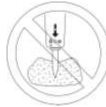
Fig 5-5 Never Drive Breaker Tool Into Material
