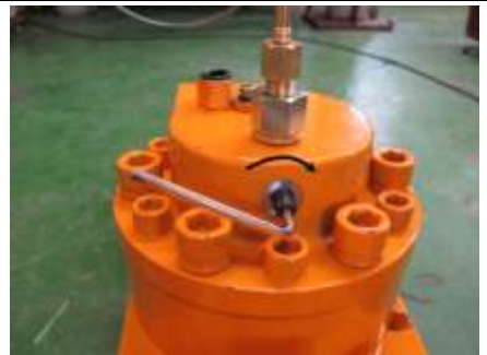
9. Close needle pin. (If equipped)
