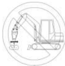
Fig 5-4 Do Not Pry With The Breaker
