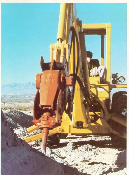
The lightweight Rapid-Ram, with its low 11 g.p.m. oil flow requirements, is well-suited for smaller backhoe/loaders.
