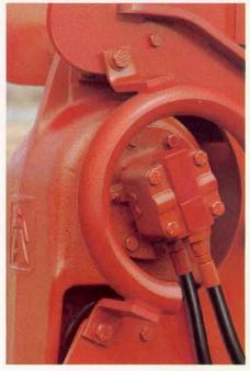
With an oil flow of just 11 g.p.m., this highly efficient hydraulic system produces 200 ft. lbs. of impact energy at a frequency of 1250 blows per minute which translates into power to break, tamp, and drive.
