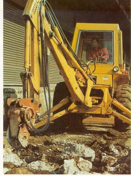
With its optional Tamper Tool, the Rapid-Ram productively drives wood, steel and aluminum sheeting, retaining walls and sea walls.
